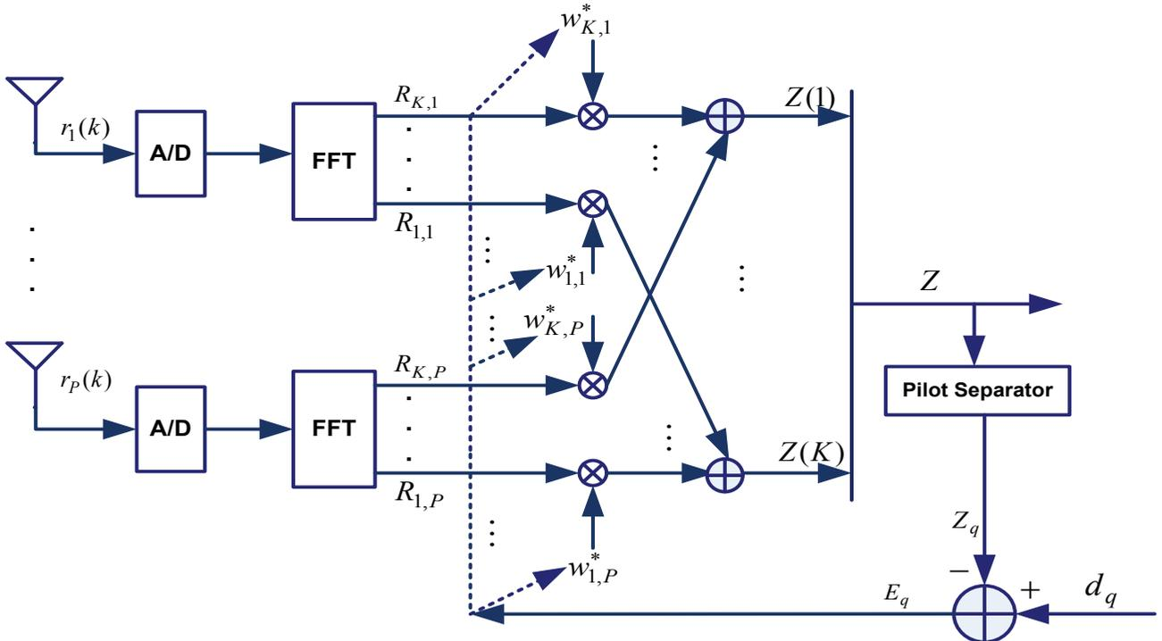
Fig. 2: Block diagram of frequency-domain (post-FFT) beamforming
